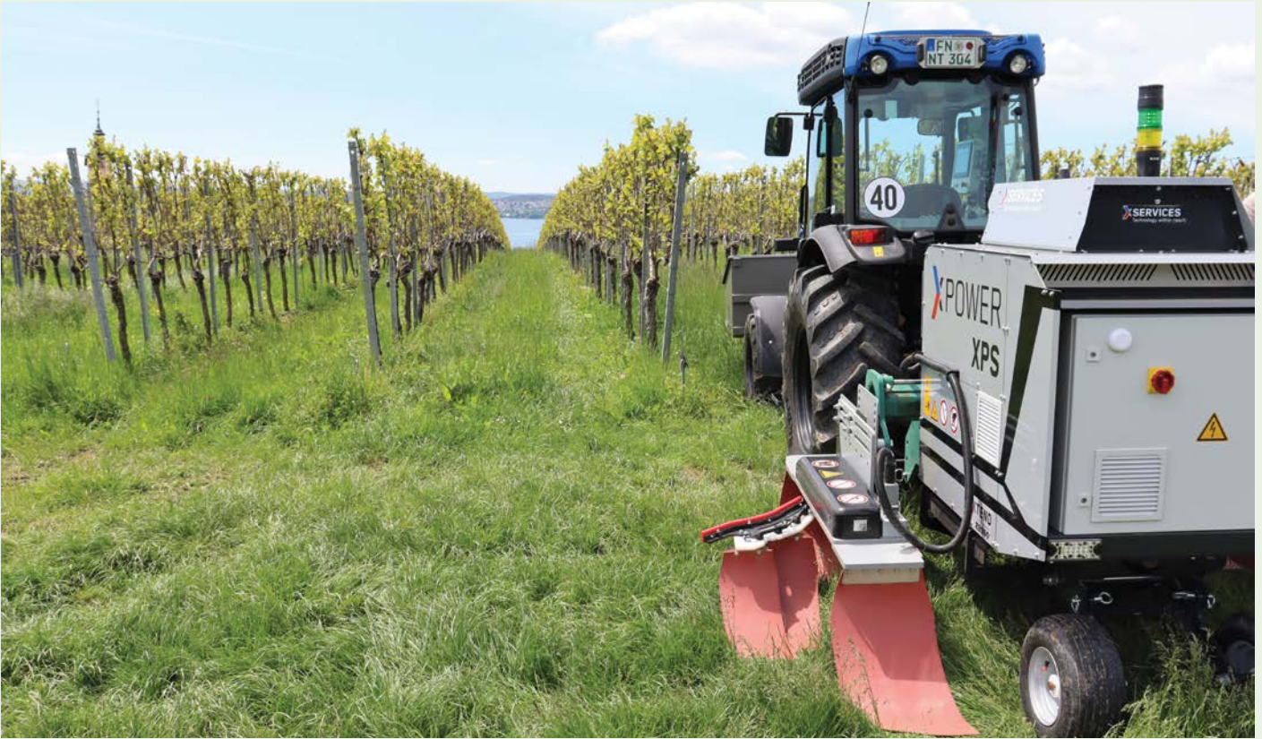
Electrical weed management (EWM) seems to be living up to its theoretical potential to be a partial replacement for glyphosate. Photo courtesy of Zasso Group AG
