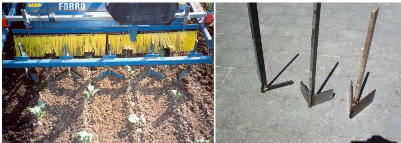
Figure 9. Mini ridgers on horizontal brush hoe (left), and different designs (right) from left to right, low profile for small ridges, large for big ridges, and low angle for high speed use.
