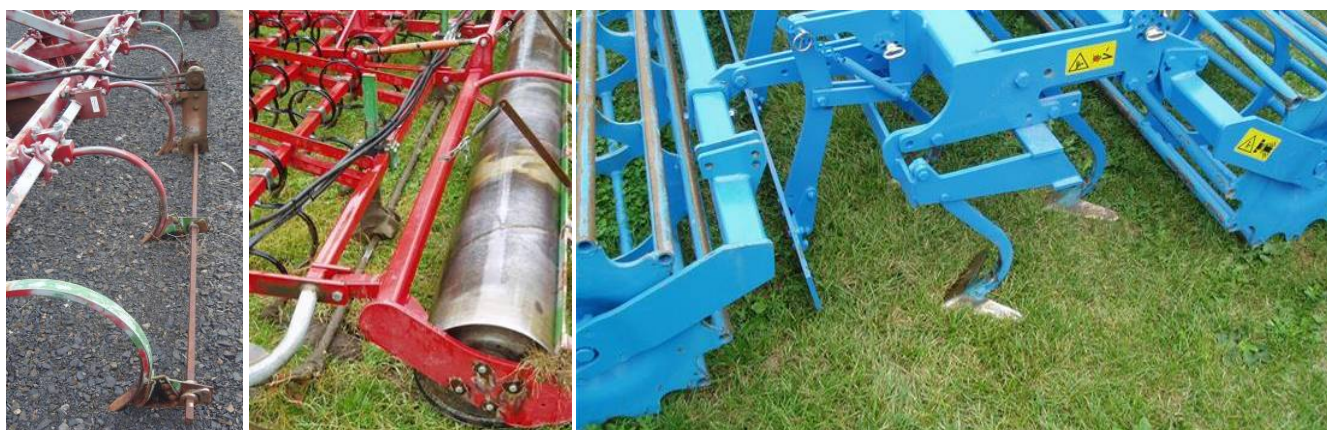
Figure 5. American rod weeder (left), false seedbed cultivator using rod weeder (middle), A-blade sweeps (right).
