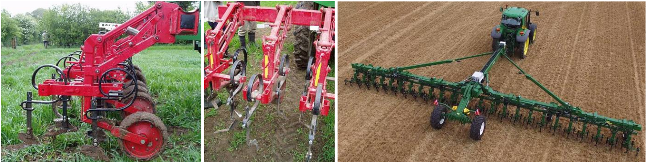
Figure 5. Parallelogram hoe consisting of a number of independent parallelogram units mounted on a toolbar. Right photo Garford Farm Machinery Ltd.
