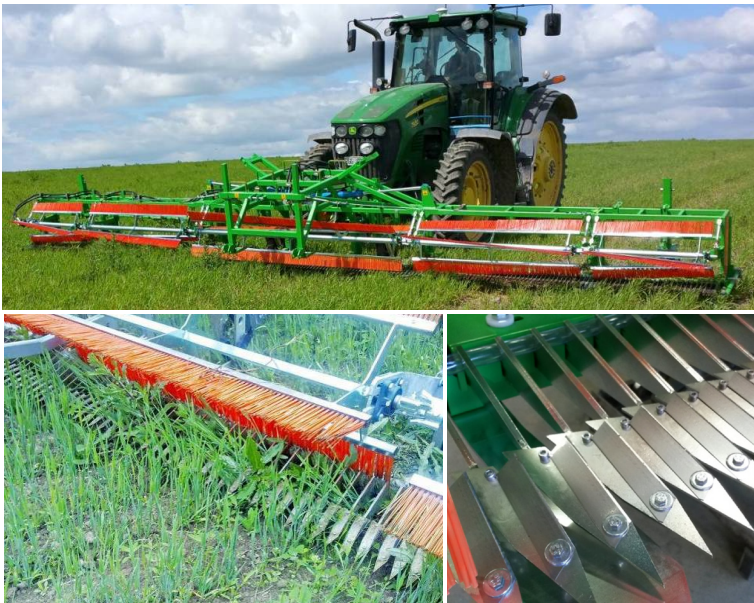
Figure 4. Combcut showing whole machine (top) weeds being cut (bottom left) adjustable knives (bottom right). Photos LyckeGård Group AB.
