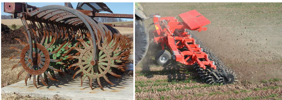
Figure 2. Spoon weeder (rotary hoe), left high residue original N. American design, right new European design. Right photo Einböck GmbH.
