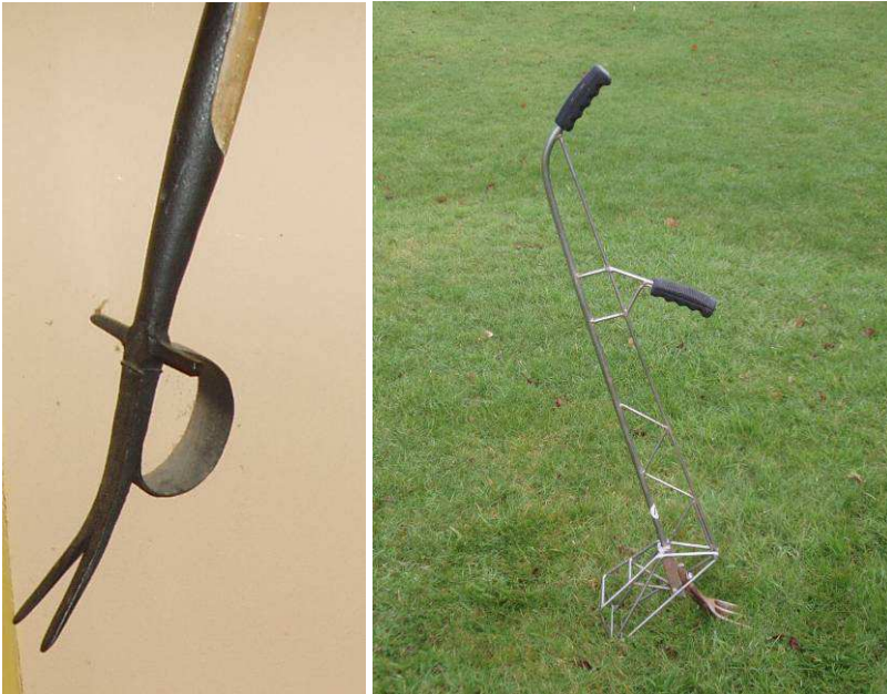
Figure 5. Traditional dock fork (left), modern ergonomic design with interchangeable heads (right) (LazyDogTools.co.uk)
