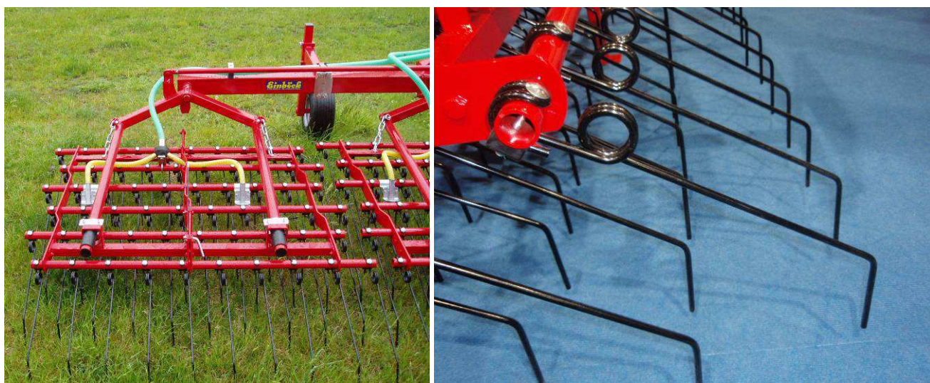
Figure 7. Spring tine weeder detail: Left, modular 'wishbone' ground following system. Right, details of spring tines.
