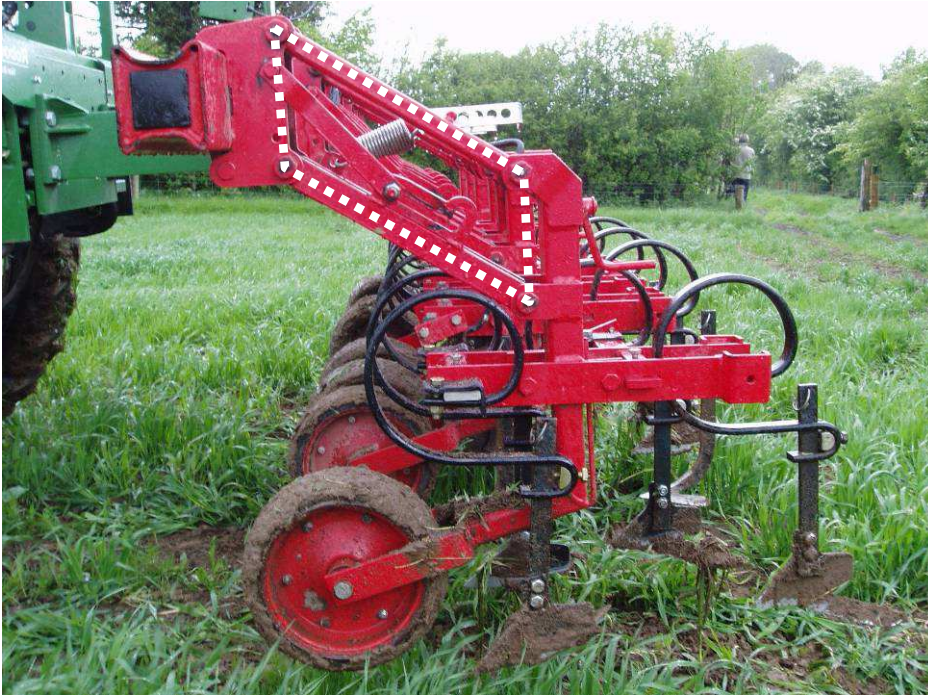
Figure 8. Modular, parallelogram interrow hoe with white dashed line indicating the parallelogram pivot system.
