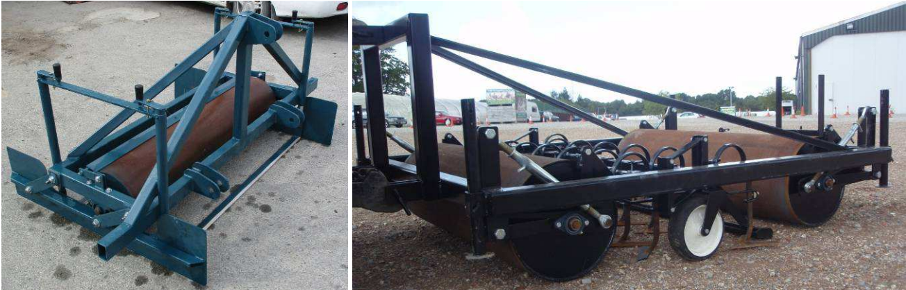
Figure 5. False seedbed cultivators. Left single roller and undercutter bar design, right, twin roller and A blade sweeps design.
