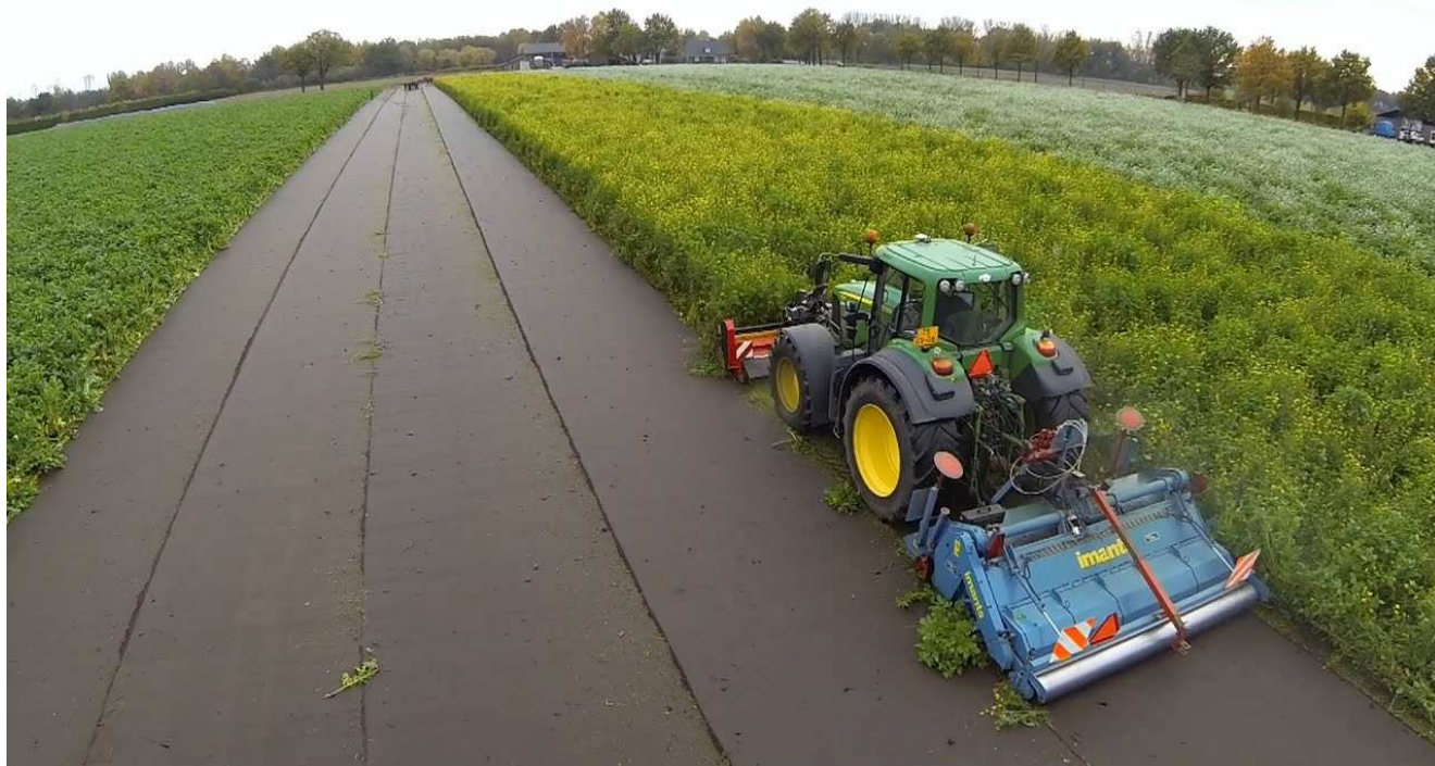
Figure 4. Single pass biofumigation system, with front mounted flail mower, rear mounted, rotary spading machine, with purpose built, powered, rear smearing roller. Credit AGROMOVIE youtu.be/SHKLFRr0GCI
