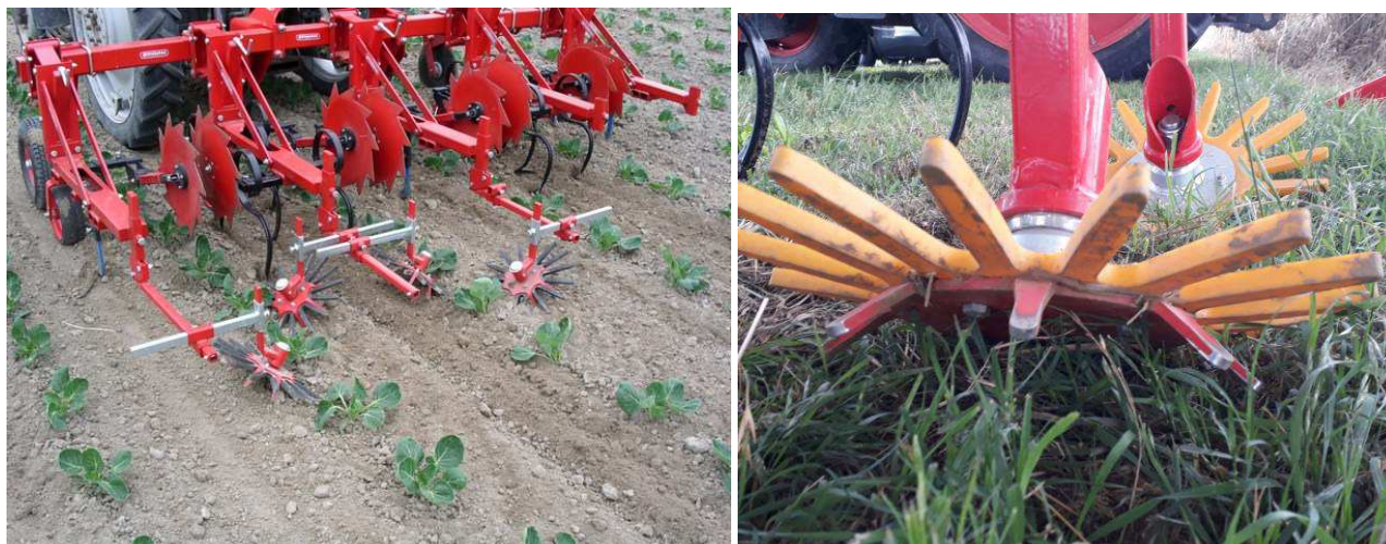
Figure 10. Finger weeders. Left weeding cabbage, right showing detail.
