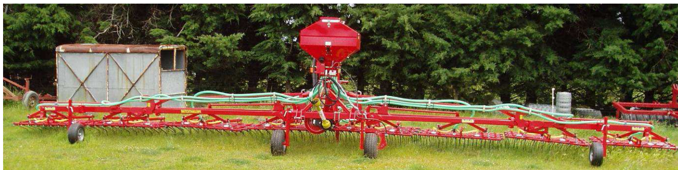
Figure 6. Large spring tine harrow with pneumatic seeder unit.
