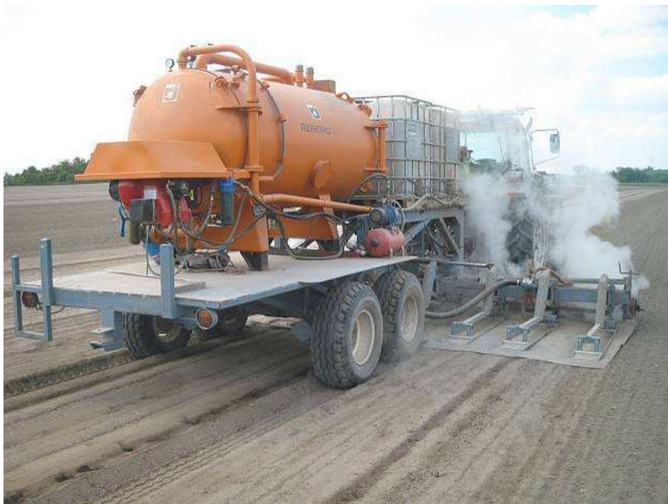
Figure 1.1: Swedish band steamer using steam injection without mechanical mixing using 600 kW steam boiler water tanks and associated equipment. Photo credits: Bo Melander.
