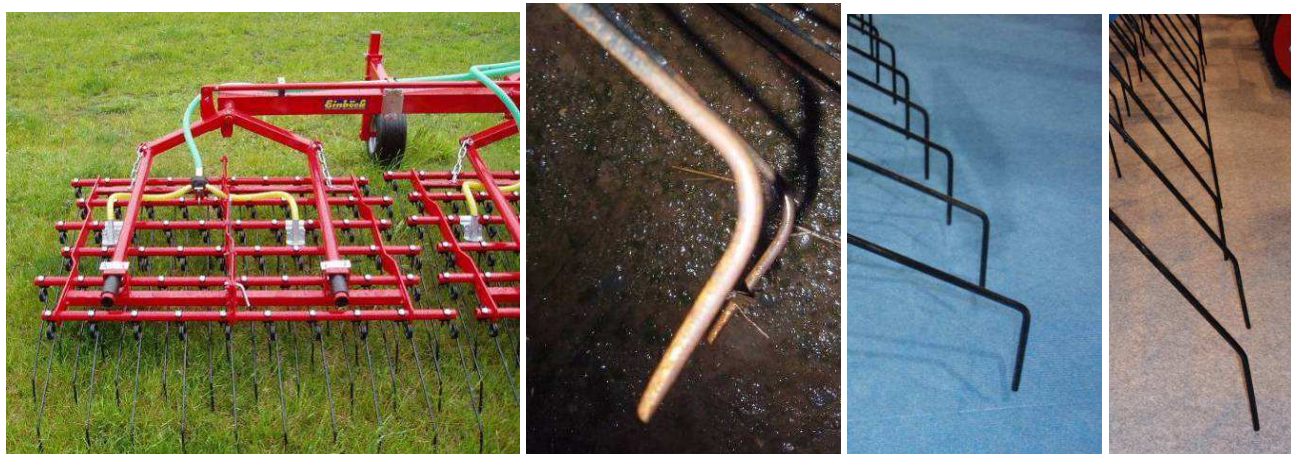
Figure 20. The modular 'wishbone' unit (left) also showing pneumatic seeder outlets, and, 90°, 45° and 15° tine angles (right three photos).
