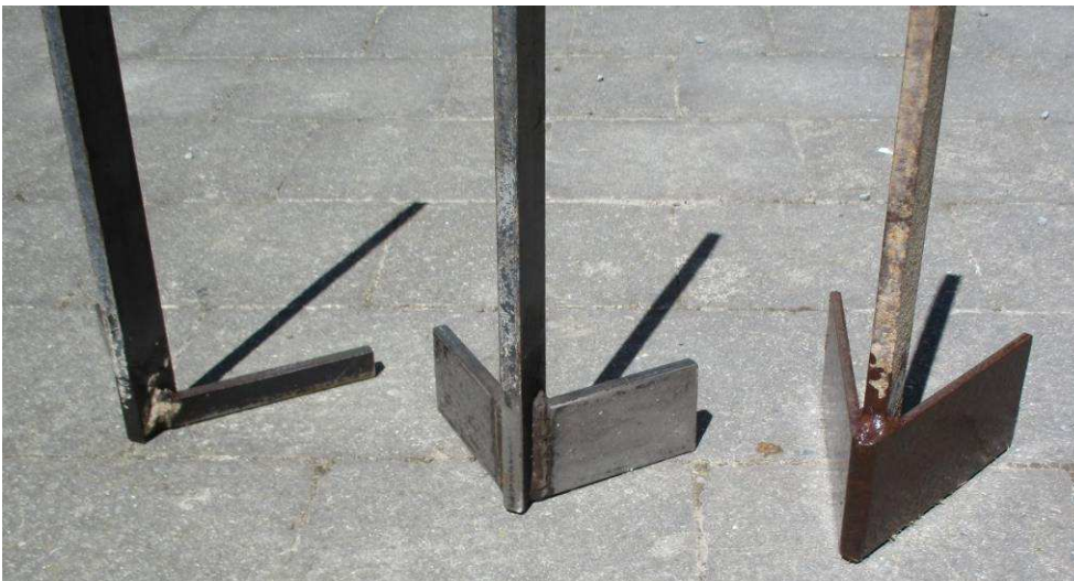
Figure 30. Three 'mini-ridgers' small ridger (left) larger ridger (middle) large high speed ridger with narrower blade angle (right).
