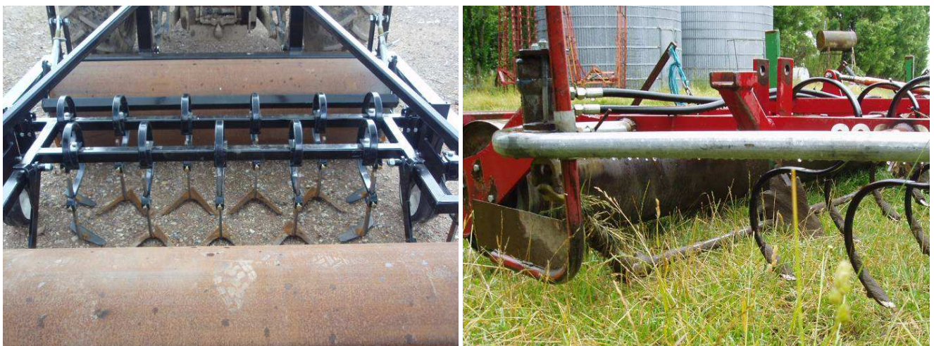
Figure 18. Twin roller and A blade hoe false seedbed tiller (left), rod weeder built into an S tine cultivator (right).
