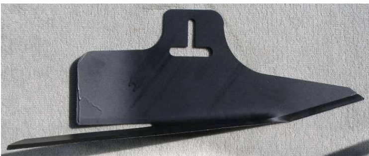
Figure 29. L blade hoe with down-cut front point, and a large 'heal' to push soil away from crop row.
