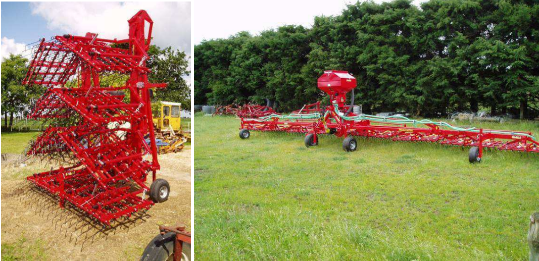
Figure 21. Large spring tine weeder, folded (left) extended (right) with pneumatic seeder attachment.
