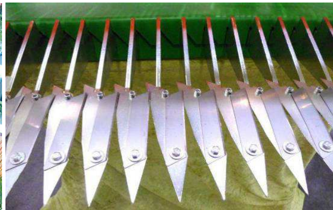
Figure 25. CombCut showing whole machine (top) weeds being cut (bottom left) adjustable knives (bottom right). Photos courtesy of LyckeGård Group AB.
