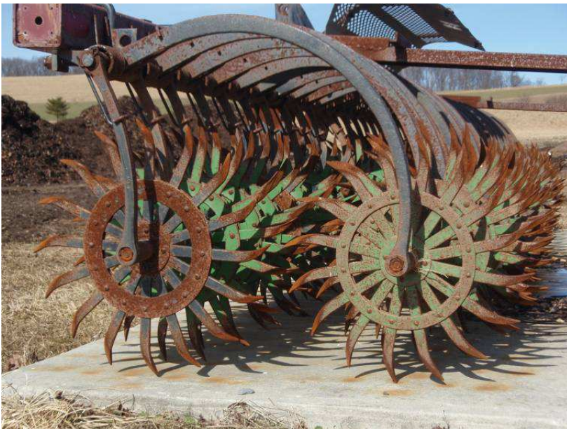
Figure 24. Spoon weeder / rotary hoe. Top, European model (photo courtesy Einböck GmbH & CoKG), bottom left, USA high residue model, bottom right spoon tips.
