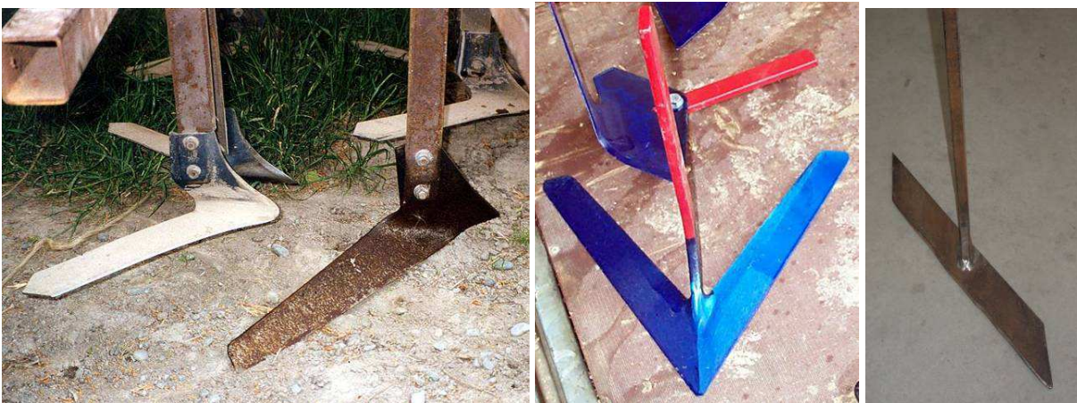
Figure 27. The three main types of horizontal knife blade hoes L blade (left) A blade (middle) T blade (right)
