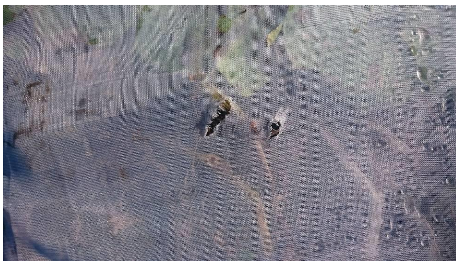
Figure 34. Hole ripped in 0.3 mm mesh in field trial - possibly by a stone from grass mowing.
