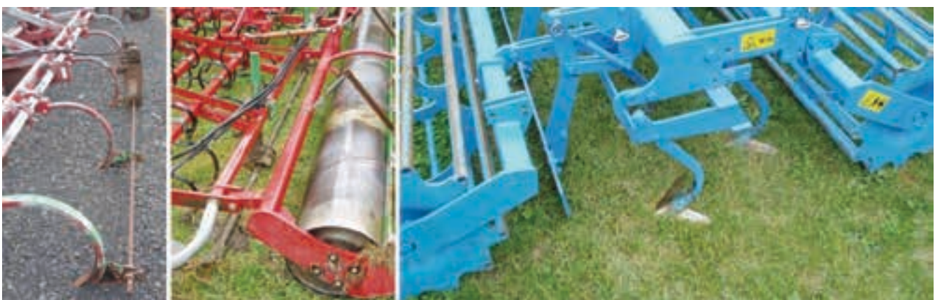
Figure 4. American rod weeder (left), false seedbed cultivator using rod weeder (middle), A-blade sweeps (right).
