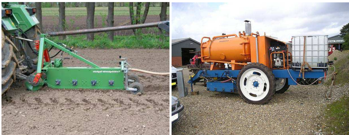
Figure 3. Danish design band steamer: left, prototype band steamer using horizontal axis rotating tines reprinted from (Kristensen et al. , 2005); right, field scale version of prototype band steamer with 900 kw pressurised steam boiler, three phase generator and water tank.
