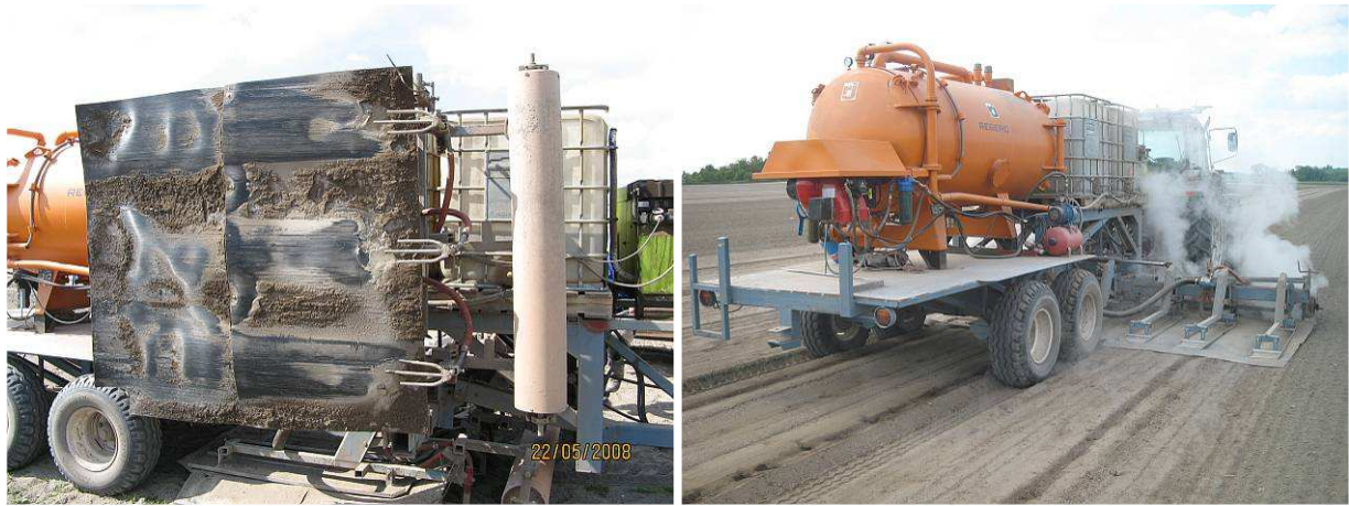
Figure 2. Swedish band steamer using steam injection without mechanical mixing using 600 kw steam boiler water tanks and associated equipment. Photo credits: Bo Melander.
