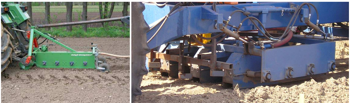
Figure 12. Danish design band steamer: left, prototype reprinted from (Kristensen et al. , 2005); right, field scale version of prototype band steamer (photo Hans Kjoeras).
