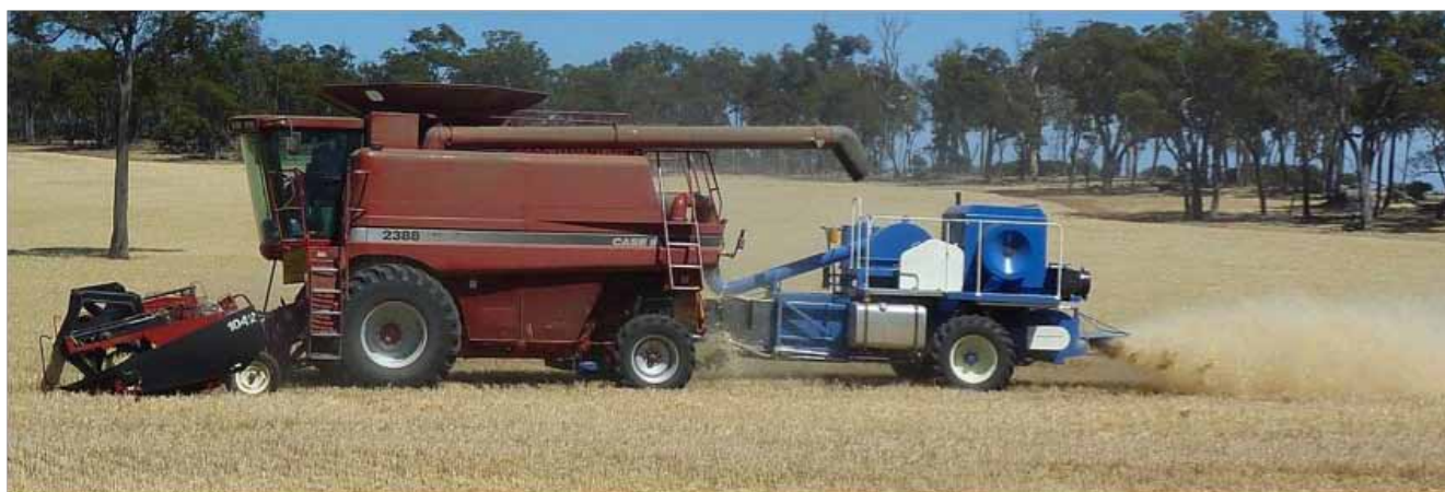
Figure 1. The 'Harrington Seed Destructor' in operation behind a header. Photo courtesy of Associate Prof Michael Walsh, The University of Western Australia.
