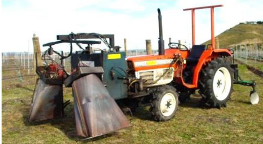
Figure A.3. Photo of the VaporJet H1200® steam weeder. © Thermal Options Ltd.
